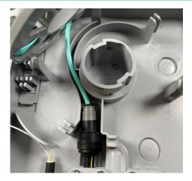
Gas block which is secured to cable sheathing can be secured inside a cable track which lead to inner cable storage tray.
